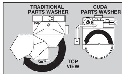
Space saving roll-in door allows easy access to the wash chamber and prevents wash solution from dripping on the shop floor.
